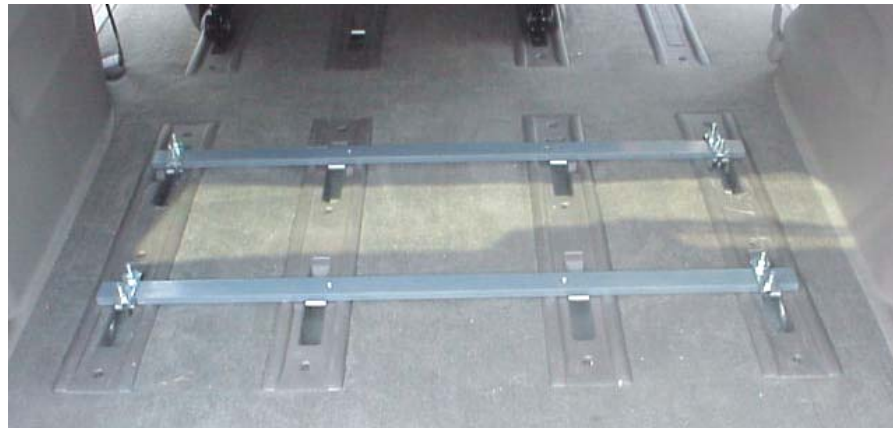
Example: Mounting Bars Installed
